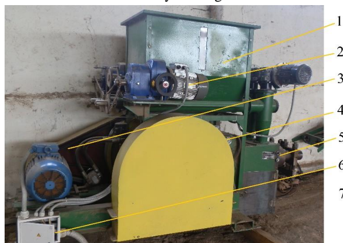
Fig. 1. Impact-mechanical briquetting press PBU-060-800 for laboratory experiments: 1 – raw material hopper-feeder; 2 – electromechanical drive of the feeder; 3 – electromechanical drive of the pressing chamber, 4 – pressing chamber; 5 – briquette forming matrix; 6 – control panel; 7 – briquette cooling line (not shown)
